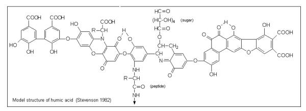
This is a molecule of Humic Acid. You can see here just one fragment of this huge molecule. These fragments are connected to each other in long chains and total weight of molecules, naturally depending on the chain length, is in the range from 35 000 to 80 000 Daltons.
