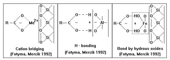
Colloid structure of Humic Acids and high degree of hydrophility of their functional groups gives them an ability for gel formation. This explains their ability to increase water holding capacity of soils. This is very important for arid regions.
